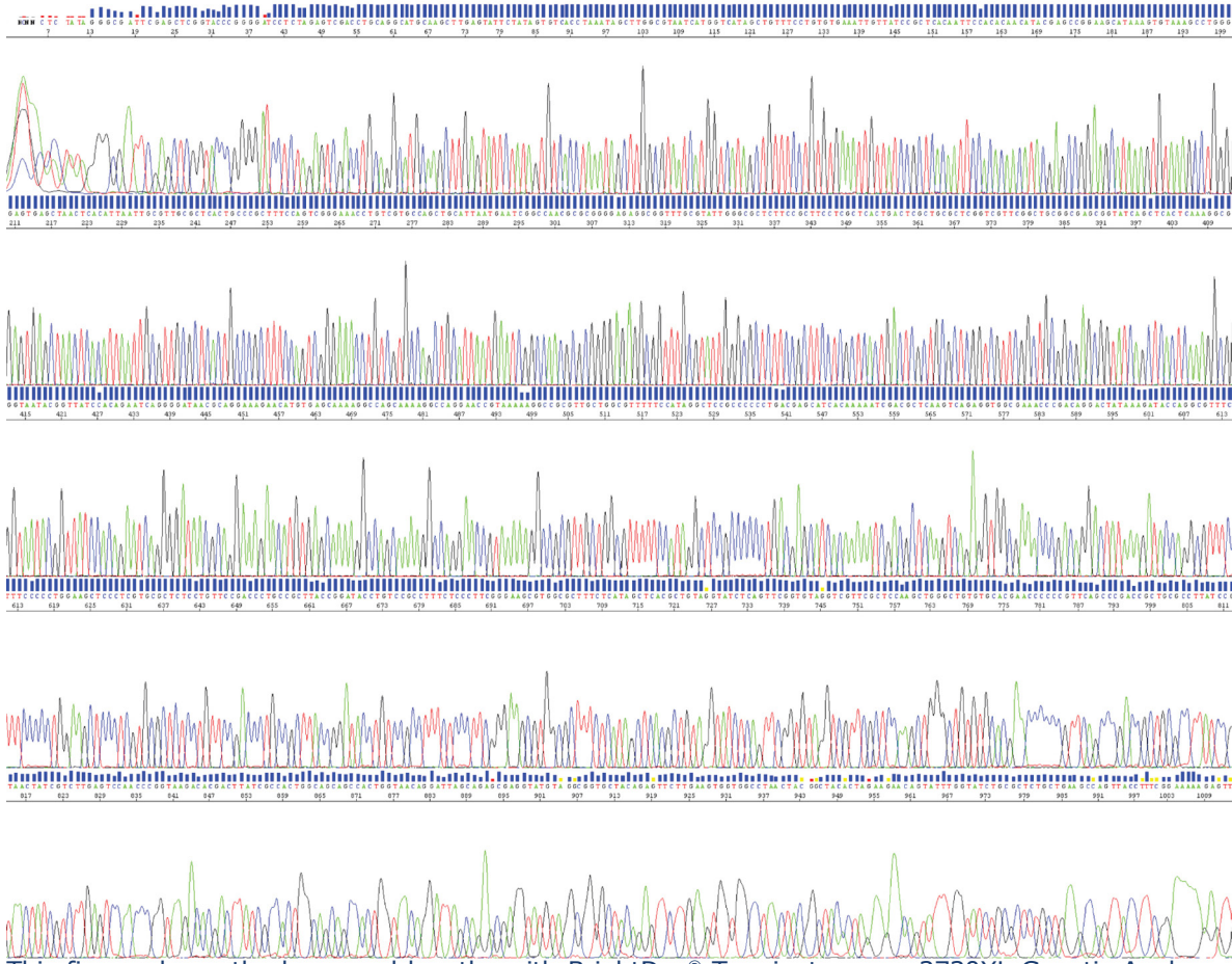
This figure shows the long read lengths with BrightDye® Terminator on a 3730XL Genetic Analyzer. pGEM control DNA was used in combination with M13 primers. Sequences were run under filter set Z.
